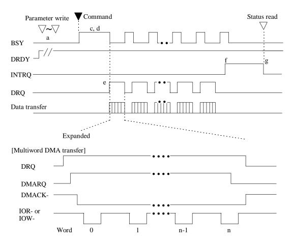
Figure 5.6 Normal DMA data transfer
